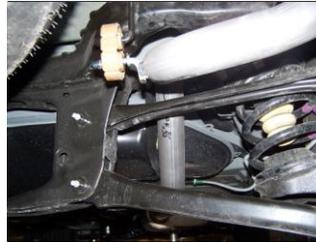
**4.** Install tailpipe #C into the muffler 1 1/2"-2" secure with clamp #F. DO NOT TIGHTEN.
