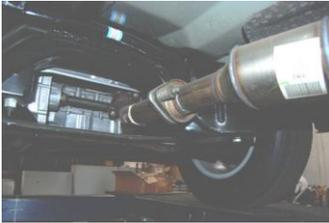
**1.** To remove the stock exhaust remove it from clamp located in front of the stock muffler. Disengage the welded hangers using WD-40 from the OEM rubber grommets. Do not damage or remove the rubber grommets as you will re-use them to mount your new system. Now, un-bolt tailpipe and remove exhaust.
