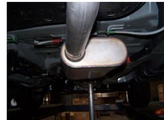
**3.** Install muffler #B onto head pipe 1 1/2"-2" with the louvers facing towards the converter. Use a jack stand to support the muffler. Use clamp #F to secure the muffler to the headpipe. DO NOT TIGHTEN.
