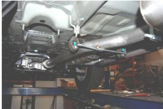
**2.** Install head pipe #A onto your existing stock front pipe and attach with clamp #F. Use a jack stand to support the converter. DO NOT TIGHTEN.
