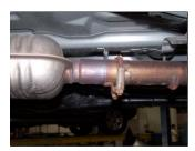
**1.** To remove the stock exhaust remove it from clamp located in front of the stock muffler. Disengage the welded hangers using WD-40 from the OEM rubber grommets. Do not damage or remove the rubber grommets as you will re-use them to mount your new system. Now, un-bolt tailpipe and remove exhaust.
