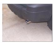
**6.** Install stainless steel tips #E. Clamp down. When you have everything in place, firmly tighten all bolts and clamps down securely. Use stainless steel cleaner and a Scotch Brite pad weekly to prevent tip from discoloration.
