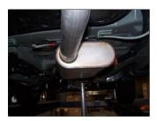
**3.** Install muffler #B onto head pipe 1½"-2" with the louvers facing towards the converter. Use a jack stand to support the muffler. Use clamp #F to secure the muffler to the headpipe. DO NOT TIGHTEN.
