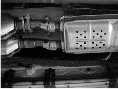
LAY OUT THE EXHAUST AND COMPARE THE PART NUMBERS TO THE MANUAL. FOR AN EASIER REMOVAL OF THE FACTORY EXHAUST CUT JUST BEHIND THE REAR MUFFLER HANGER AND REMOVE THE TAIL PIPE. THEN UN-BOLT THE FLANGE AND CLAMP IN FRONT OF THE STOCK MUFFLER. **YOU WILL RE-USE THE DRIVERSIDE FLANGE GASKET, BOLTS.** LEAVE ALL FACTORY RUBBER GROMMETS IN PLACE.
