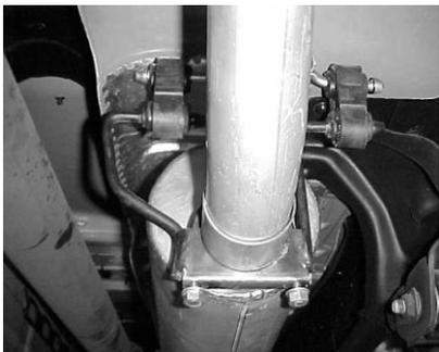
INSTALL REAR MUFFLER HANGER # D ON TO THE OUTLET OF THE MUFFLER AND INSERT WELDED RODS INTO RUBBER GROMMET. THE VERTICAL ROD'S ON THE HANGER WILL BE FACING TOWARDS THE PASSENGER SIDE. DO NOT TIGHTEN.
