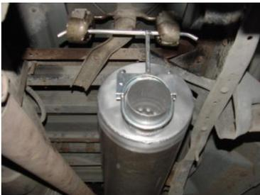
INSTALL MUFFLER #B ONTO HEADPIPE #A 1-1/2" TO 2". USE A JACKSTAND TO SUPPORT MUFFLER. SECURE MUFFLER TO HEADPIPE WITH CLAMP #I. DO NOT TIGHTEN. INSTALL HANGER #G ONTO OUTLET OF MUFFLER AND INSERT HANGERS INTO RUBBER GROMMETS. MUFFLER INLET IS LOOKING INTO THE LOUVERS.
