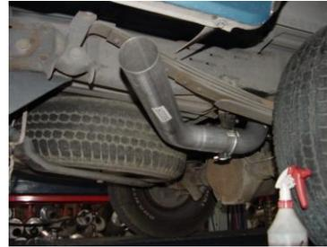
INSTALL THE TURNOUT PIPE #D ONTO THE TAILPIPE #C. SECURE TOGETHER WITH CLAMP #I. DO NOT TIGHTEN. ROLL THE TURNOUT PIPE UNTIL IT IS AT THE CORRECT LEVEL FOR YOUR TRUCK.
