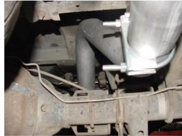
INSTALL THE OVERAXLE TAILPIPE #C INTO THE MUFFLER 1-1/2" TO 2". SECURE TO THE MUFFLER USING CLAMP #I. SLIDE HANGER #H ONTO THE END OF THE TAILPIPE AND INSERT HANGER INTO RUBBER GROMMET. DO NOT TIGHTEN.
