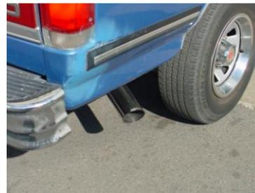
INSTALL THE STAINLESS TIP. TO CLEAN TIP USE ANY STAINLESS CLEANER AND A SCOTCH BRITE PAD. NOW GO BACK AND TIGHTEN ALL CLAMPS STARTING FROM THE FRONT AND WORKING BACK.
