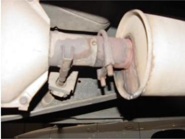
LAY OUT THE EXHAUST ON THE FLOOR SO IT LOOKS LIKE THE DRAWING AND COMPARE PARTS TO THE MANUAL. TO REMOVE STOCK EXHAUST UN-BOLT THE CLAMP LOCATED JUST BEHIND THE CATALYTIC CONVERTER. USE JACK STANDS TO SUPPORT THE CONVERTER. LEAVE ALL RUBBER GROMMETS IN PLACE. FOR EASIER REMOVAL USE WD-40 ON HANGERS.
