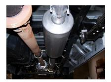
**3.** INSTALL MUFFLER # B. THROUGH BAND CLAMP THEN SLIDE ONTO HEADPIPE 11/2" TO 2". USE CLAMP #E TO SECURE MUFFLER TO HEADPIPE.
