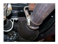
2. To remove your stock exhaust, remove the clamp located just behind the converter. Disengage the welded hangers from the OEM rubber grommets. Use WD-40 to aid in the process. Do not damage or remove the rubber grommets as you will re-use them. Now, cut off tailpipe and remove exhaust.
