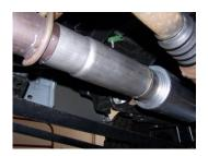
3. Install headpipe #A onto your existing stock front pipe and attach with clamp #F. Insert welded hanger into rubber grommet.
