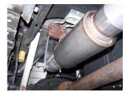
4. Install muffler #B onto headpipe #A 1.5"-2" with the louvers facing towards the tailpipe. Use clamp #G to secure the muffler to the headpipe. Do not tighten. Muffler outlet is looking into the louvers.
