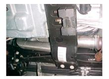
INSTALL PIPE #J ONTO PIPE #K. USE CLAMP #H TO SECURE PIPES TOGETHER. DO NOT TIGHTEN.
