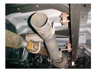
Install head pipe # A on to your existing stock down pipe and line up the notch. Then secure with clamp # H. Insert hangers into rubber grommets. Do not tighten.
