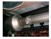
1. To remove the stock exhaust disengage the welded hangers using WD-40 from the OEM rubber grommets. Do not damage or remove the rubber grommets as you will re-use them to mount your new system. Now, cut off tailpipe and remove exhaust.
