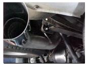
**7.** Install the exit pipe #D onto the over axle tailpipe and secure with clamp #G. DO NOT TIGHTEN. Insert welded hanger into rubber grommet
