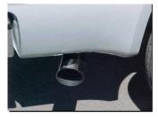
**8.** Install stainless steel tip #E. Clamp down. When you have everything in place, firmly tighten all bolts and clamps down securely. Use stainless steel cleaner and a Scotch Brite pad weekly to prevent tip from discoloration.
