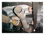
**2.** Install headpipe #A onto your catalytic converter and attach with clamp #H. Use a jack stand to support the converter. DO NOT TIGHTEN. Insert welded hangers into rubber grommets.
