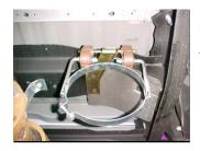
**3.** Install band clamp #F into rubber grommets located above the axle and attach bolt kit #I. DO NOT TIGHTEN.
