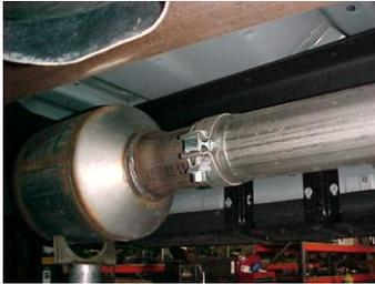
Lay out the exhaust on the floor so it looks like the drawing and compare parts with manual. To remove the stock exhaust remove it from the clamp located just behind the catalytic converter. Cut off your stock tailpipe for easier removal. Leave all rubber grommets in place. Use WD-40 to aid in removal of exhaust and hangers.
