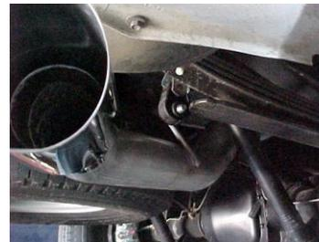
Install exit pipe # D onto over axle pipe. Then insert welded hanger into rubber grommet. Use clamp # G to secure pipes together.
