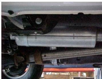
Install muffer # B onto head pipe # A 1-1/2" to 2" with the louvers facing towards the converter. Use a jack stand to support the muffer. Use clamp # G to secure the muffer to the head pipe. Do not tighten. Muffer inlet is looking into the louvers.
