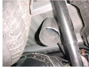
Install the over axle tailpipe # C into the muffer 1-1/2" to 2". Secure to the muffer using clamp # G. Do not tighten.
