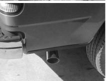
Slip tailpipe #C into muffler no less than 1-1/2" and no more than 2" and attach with hanger # H and clamp # G to connect 10" hanger to rear of tailpipe. DO NOT TIGHTEN
