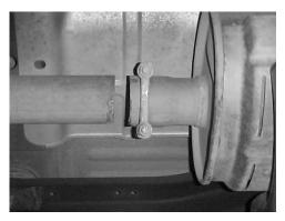
Cut stock exhaust approximately 4" in front of muffler body removing the alignment pin. Leave all rubber grommets in place.
