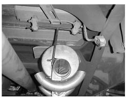
Slip headpipe #A into Gibson muffler inlet no less than 1-1/2" and no more than 2". Slip both onto stock headpipe no less than 1-1/2" and no more than 2", and install rear muffler T-hanger #H. Bolts on T-hanger will aim towards drivers side. Make clamps snug but **DO NOT TIGHTEN** at this time. Rear muffler clocking is at approximately 6 o'clock. Muffler inlet is looking into louvers.
