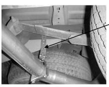
Install rear tailpipe hanger #I. Measure from rear of frame 21" forward to slotted hole. Place bolt with large washer from inside frame out. Put 10" hanger on outside of frame. Bolt through top hole, put lock washer and nut on and tighten. End of hanger swivels so it can be adjusted for 3" clamp.
