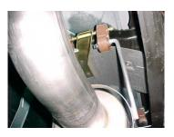
Install band clamp # G into rubber grommets located just above the axle. Do not tighten. Attach with bolt kit #J.
