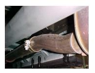
Lay out the exhaust on the floor so it looks like the drawing and compare parts with manual. To remove the stock exhaust remove it from the clamp located just in front of the muffler.
