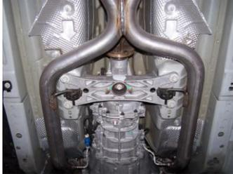
4. Now install the Gibson X Pipe by bolting it up to the stock manifolds using the bolt kit provided. Do not tighten the flanges at the manifolds.
