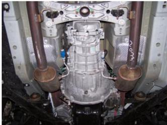
3. Now disconnect 2 sensors on stock h-pipe with a 22mm wrench. Once you have done that, then unbolt the flanges at the stock manifolds and slide h-pipe out. Save all stock hardware and clamps. You will re-use them later.
