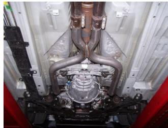
7. Now firmly tighten all bolts and clamps. Inspect all fasteners after 25-50 miles of operation and re-tighten as necessary.
