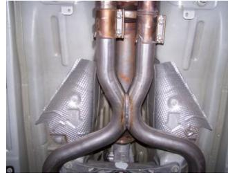
6. Now slide the X Pipe and the tailpipes together and re-clamp them using your stock clamps.
