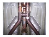
3. Loosen up the 2 clamps in the middle of the vehicle and slide them over the tailpipes. Now separate both tailpipes from mufflers and slide them out. Next remove the stock mufflers by sliding them out of the stock rubber grommets.
