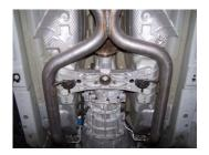
3. Now disconnect all 3 sensors on stock h-pipe with a 22mm wrench. Once vou have done that, then unbolt the flanges at the stock manifolds and slide h-pipe out of rubber grommets. Save all stock hardware and clamps. You will re-use them later.
