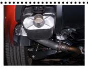
3. Install driver side muffler assembly #A onto stock flange using bolt kit #C. Use a jack stand to support the muffler to insert welded hangers into rubber grommets. Insert clips onto hangers.
