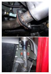
**3.** Install passenger side muffler assembly #A onto stock flange using bolt kit #C. Use a jack stand to support the muffler to insert welded hangers into rubber grommets. Insert clips onto hangers.
