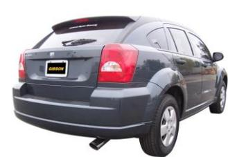
7. Install stainless steel tip. Clamp down. When you have everything in place, firmly tighten all bolts and clamps down securely. Use stainless steel cleaner and a Scotch Brite pad weekly to prevent tip from discoloration. Inspect all fasteners after 25-50 miles of operation and re-tighten as necessary.
