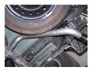
6. Install the over axle tailpipe #C into the muffler 1.5-2". Use clamp #E to secure tailpipe to muffler. Do not tighten. Insert welded hanger into rubber grommet.
