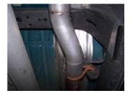
3. Install headpipe #A onto your existing stock headpipe and secure with clamp #E. Use a jack stand to support the converter.
