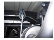
5. Slide band clamp #F onto muffler #B and attach with bolt kit #G. Do not tighten. Insert hangers into rubber grommets.
