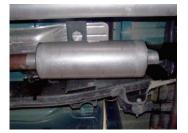
4. Install muffler #B onto headpipe #A 1.5-2" with the louvers facing towards the converter. Use a jack stand to support the muffler. Use clamp #E to secure the muffler to the headpipe. Do not tighten. Muffler inlet is looking into the louvers.
