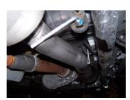
5. Install muffler #B onto head pipe #A 11/2"-2" with the louvers facing towards the converter. Use a jack stand to support the muffler. Use clamp #D to secure the muffler to the head pipe. Do not tighten. Muffler inlet is looking into the louvers.
