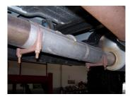
3. Remove the rest of your stock exhaust from the 2nd clamp located in front of your stock muffler.
