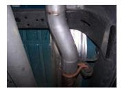
**2.** Install head pipe #A onto your existing stock front pipe and attach with clamp #E. Use a jack stand to support the converter.
