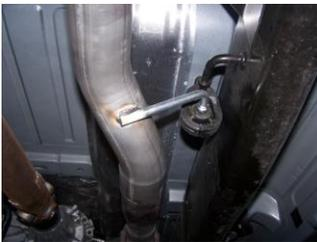
**2.** Install head pipe #A onto your existing stock front pipe and attach with clamp #F. Use a jack stand to support the converter. Insert welded hanger into rubber grommet.
