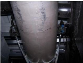
**4.** Slide band clamp #G onto muffler and attach with bolt kit #H. **DO NOT TIGHTEN.** Insert hangers into rubber grommets.
