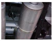
SLIDE BAND CLAMP #G ONTO MUFFLER #B. INSERT HANGERS INTO RUBBER GROMMETS.
