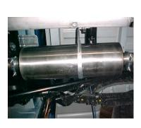
**INSTALL MUFFLER #B ONTO** HEADPIPE #A 1-1/2" TO 2" WITH THE LOUVERS FACING TOWARDS THE CONVERTER. USE A JACK STAND TO SUPPORT THE MUFFLER. USE CLAMP #F TO SECURE THE MUFFLER TO THE HEADPIPE. DO NOT TIGHTEN. MUFFLER INLET IS LOOKING INTO THE LOUVERS.
