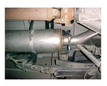
SLIDE BAND CLAMP #G ONTO MUFFLER #B. **INSERT HANGERS INTO** RUBBER GROMMETS. USE BOLT KIT #H TO TIGHTEN UP BAND CLAMP.
