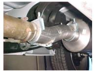
INSTALL EXIT PIPE #D OVERAXLE PIPE, ROLL TURNOUT PIPE UNTIL YOU HAVE IT AT THE CORRECT ANGLE FOR YOUR TRUCK AND CONNECT WITH CLAMP #F. BUT DO NOT TIGHTEN.
