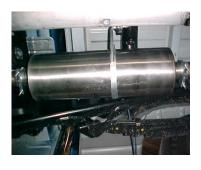
**INSTALL MUFFLER #B ONTO** HEADPIPE #A 1-1/2" TO 2" WITH THE LOUVERS FACING TOWARDS THE CONVERTER. USE A JACK STAND TO SUPPORT THE MUFFLER. USE CLAMP #F TO SECURE THE MUFFLER TO THE HEADPIPE. DO NOT TIGHTEN.
