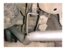
NEXT, INSTALL REAR MUFFLER HANGER #G ONTO TAILPIPE. INSERT HANGERS INTO RUBBER GROMMET.
