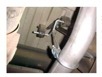
INSTALL THE OVERAXLE TAILPIPE #C TO THE MUFFLER. USE CLAMP #E TO SECURE PIPE TO MUFFLER. BUT DO NOT TIGHTEN.
