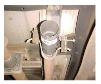
UNCLAMP EXHAUST IN FRONT OF STOCK MUFFLER. IF YOU HAVE AN EXTENSION PIPE BETWEEN THE CONVERTER AND MUFFLER- DO NOT REMOVE! LEAVE ALL RUBBER GROMMETS IN PLACE. INSTALL HANGERS AS PROVIDED. INSTALL HEADPIPE #A ONTO YOUR EXISTING STOCK FRONT PIPE AND CONNECT WITH CLAMP #F. USE JACKSTAND TO SUPPORT THE CONVERTER.
