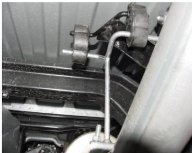
INSTALL HANGER #H AS PROVIDED. VERTICAL ROD ON HANGER #H SHOULD BE TO THE LEFT OF THE CENTER OF THE MUFFLER.
