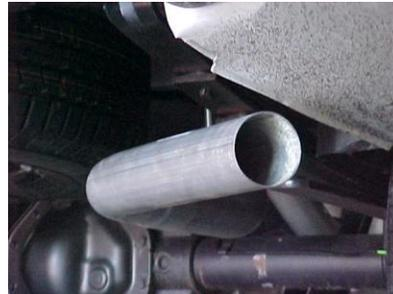
INSTALL EXIT PIPE #D OVERAXLE PIPE. ROLL TURNOUT PIPE UNTIL YOU HAVE IT AT THE CORRECT ANGLE FOR YOUR TRUCK AND CONNECT WITH CLAMP #F. DO NOT TIGHTEN.
