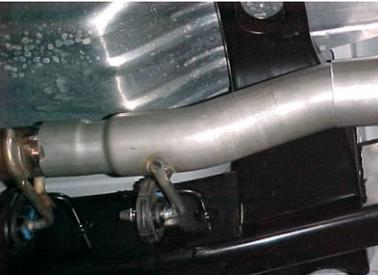
INSTALL HEADPIPE #A ONTO YOUR EXISTING STOCK FRONT PIPE AND SECURE WITH CLAMP #G. USE A JACKSTAND TO SUPPORT THE CONVERTER. INSERT WELDED HANGER INTO RUBBER GROMMET. USE WD-40 TO AID IN REMOVAL OF EXHAUST AND HANGERS. CUT OFF YOUR TAIL PIPE.
