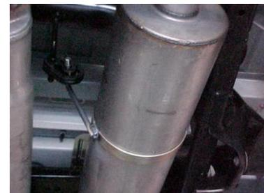
SLIDE BAND CLAMP #H ONTO MUFFLER #B. INSERT HANGERS INTO RUBBER GROMMETS AND ATTACH WITH #I.
