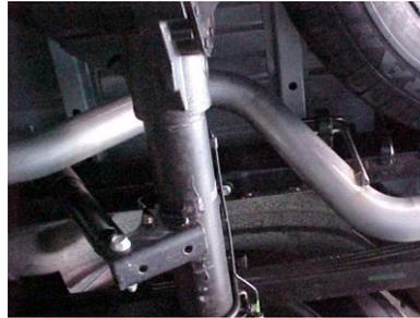
INSTALL THE OVERAXLE TAILPIPE #C INTO THE MUFFLER 1-1/2" TO 2". INSERT WELDED HANGER INTO RUBBER GROMMET. USE CLAMP #F TO SECURE TAILPIPE TO THE MUFFLER. DO NOT TIGHTEN.
