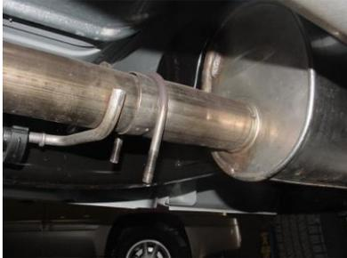
LAY OUT THE EXHAUST ON THE FLOOR SO IT LOOKS LIKE THE DRAWING AND COMPARE PARTS TO THE MANUAL. TO REMOVE THE STOCK EXHAUST UN-CLAMP IT JUST IN FRONT OF THE MUFFLER. YOU MAY NEED TO HEAT IT UP FOR EASIER REMOVAL. LEAVE ALL RUBBER GROMMETS IN PLACE.
