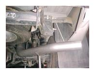
Install the turnout pipe # C on to the tailpipe. Insert welded hanger into rubber grommet. Secure together with clamp # G . Do not tighten. Roll the exit pipe until it is at the correct angle for your truck.
