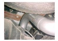
Install the over axle tailpipe # B into the muffler 1-1/2" to 2". Secure to the muffler using clamp # F. Do not tighten. Insert hanger into rubber grommet.
