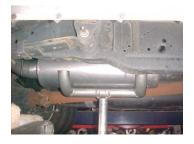
Install muffler # A on to your existing stock front pipe and secure with clamp # E. Make sure to line up the notch. Insert welded hanger into rubber grommet. Do not tighten. Muffler inlet is looking into the louvers.
