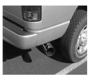
Install band clamp #I onto muffler with hanger rods facing forward and insert hangers into rubber grommet. Do not tighten.
