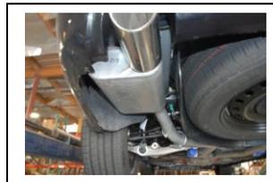
3. Next install your driver and passenger side muffler assembly's. Insert welded hangers into rubber grommets adjust assembly's. Use clamps #C to secure
