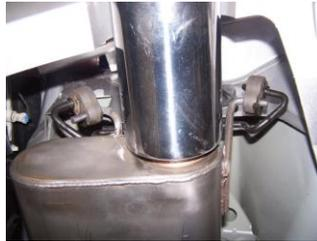
**3.** To install passenger side muffler assembly #B, insert welded hangers into rubber grommets. Use clamp #C to secure to stock tailpipe. Adjust muffler assembly to best suit your vehicle and tighten clamp.
