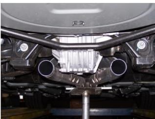
**1.** To remove the stock exhaust, cut off stock muffler just after the 90 degree bend just behind the rear axle as shown in the pictures. Disengage welded hangers from rubber grommets to remove stock muffler. DO NOT damage rubber grommets they will be reused to install the new exhaust.
