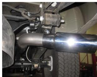
7. Install stainless steel tip. Clamp down. When you have everything in place, firmly tighten all bolts and clamps down securely. Inspect all fasteners after 25-50 miles of operation and re-tighten as necessary.
