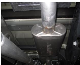
4. Install muffler #B onto headpipe #A 1.5-2" with louvers facing towards the converter. Use a jack stand to support the muffler
