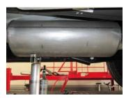
4. Install muffler #B onto head pipe  $1\frac{1}{2}$ "-2" with the louvers facing towards the converter. Use a jack stand to support the muffler. Use clamp #F to secure the muffler to the headpipe. DO NOT TIGHTEN. Muffler inlet is looking into louvers.
