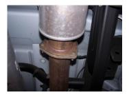
2. To remove your stock exhaust, unbolt it at the 3-bolt flange located in front of your stock muffler. Disengage the welded hangers from the rubber grommets. Use WD-40 to aid in this process. Do not damage or remove the rubber grommets as you will reuse them to mount the new system. Now, cut off the tailpipe and remove the exhaust.
