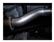
3. Install headpipe #A onto stock flange. Use bolt kit #G to attach. Do not tighten.
