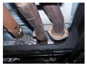
2. To remove the stock exhaust, remove it from the clamp on the driver side & flange on the passenger side located in front of the stock muffler. Disengage the welded hangers using WD-40 from the OEM rubber grommets. Do not damage or remove the rubber grommets as you will reuse them to mount your new system. Now, cut off tailpipe and remove exhaust.
