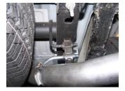
**5.** Next, insert the welded hanger from over axle pipe into rubber grommet. Rotate pipe for proper angle and clearance.
