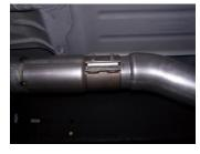
Install head pipe #B onto down pipe using factory clamp to secure. DO NOT TIGHTEN. Insert hangers into rubber grommets.
