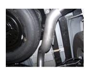
Install stainless steel tip. Clamp down.
