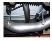
Install head pipe #A onto your factory down pipe using factory clamp to secure. DO NOT TIGHTEN. Insert hangers into rubber grommets.
