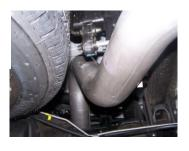
Install the overaxle tail pipe #D into the muffler 1½-2". Secure to muffler using clamp #F. DO NOT TIGHTEN.
