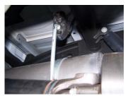
Install muffler #C onto head pipe 1½-2", with louvers facing forward. Use a jack stand to support the muffler. Use clamp #F to secure the muffler to the headpipe. Muffler inlet is looking into the louvers. Install band clamp #E to support muffler, insert hanger into rubber grommet. Use bolt kit #H to secure band clamp to muffler. DO NOT TIGHTEN.
