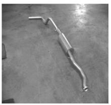
TO REMOVE EXHAUST UNBOLT THE 2 BOLT FLANGE LOCATED JUST BEHIND THE CATALITIC CONVERTER. YOU WILL RE-USE STOCK FLANGE BOLTS. NOW CUT OFF YOUR STOCK TAILPIPE JUST BEHIND THE MUFFLER AND REMOVE. LEAVE ALL RUBBER GROMMETS ON THE HANGER. USE WD-40 TO AID IN THE REMOVAL OF EXHAUST AND HANGERS.
