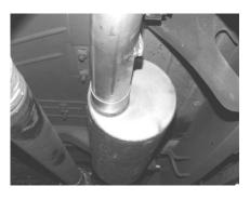
INSTALL MUFFLER #B ONTO HEADPIPE 1-1/2" TO 2" WITH INLET TOWARDS THE MOTOR. OUTLET SHOULD BE AT THE 9 O'CLOCK POSITION USE CLAMP #F TO SECURE MUFFLER TO THE HEADPIPE. USE A JACKSTAND TO SUPPORT MUFFLER. DO NOT TIGHTEN. MUFFLER INLET IS LOOKING INTO LOUVERS.
