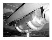
INSTALL MUFFLER #B ONTO HEADPIPE 1-1/2" TO 2" WITH THE LOUVERS FACING TOWARDS THE CONVERTER. USE A JACK STAND TO SUPPORT THE MUFFLER. USE CLAMP #F TO SECURE THE MUFFLER TO THE HEADPIPE. DO NOT TIGHTEN. MUFFLER INLET IS LOOKING INTO THE LOUVERS. OUTLET SHOULD BE AT THE 6 O'CLOCK POSITION.
