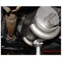
NEXT INSTALL MUFFLER #C. SLIDE IT ONTO HEADPIPE 1-1/2" TO 2". INLET OF MUFFLER SHOULD FACE TOWARDS THE MOTOR. ATTACH WITH CLAMP # F.
