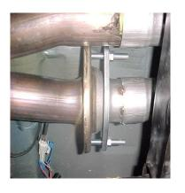
INSTALL PASS. SIDE HEADPIPE # A USING HARDWARE # H. DO NOT TIGHTEN. INSERT HANGER INTO RUBBER GROMMET, NEXT SLIP DR. SIDE HEADPIPE # B ONTO FACTORY PIPE USE CLAMP # F TO SECURE. DO NOT TIGHTEN.
