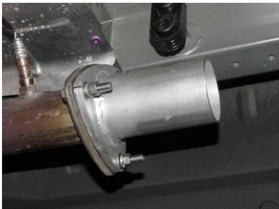
INSTALL HEADPIPE #A USING BOLT KIT #H AND FLANGE GASKET #G AND RE-USING FACTORY BOLTS. DO NOT TIGHTEN.
