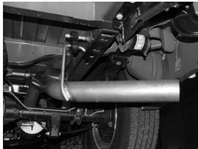
SLIDE OVERAXLE TAILPIPE #E INTO THE OUTLET OF THE MUFFLER 1 1/2" TO 2". INSERT WELDED HANGER INTO RUBBER GROMMET AND CLAMP DOWN USING HANGER # D.
