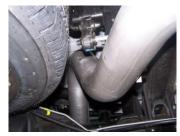
Install the over axle tail pipe #D into the muffler  $1\frac{1}{2}-2^{"}$ . Secure to muffler using clamp #F. DO NOT TIGHTEN.
