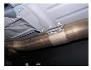
Lay out the exhaust on the floor so it looks like the drawing and compare parts with manual. To remove the stock exhaust unclamp it just in front of muffler. Save factory clamp. Leave all rubber grommets in place. Use WD-40 to aid in removal of exhaust and hangers.
