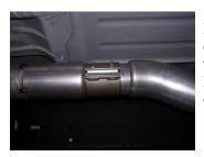
Install head pipe #B onto down pipe using factory clamp to secure. DO NOT TIGHTEN. Insert hanger into rubber grommet.
