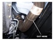
Cut factory down pipe just before converter (see picture). Then unclamp it from the turbo and remove. Save clamp it will be reused.
