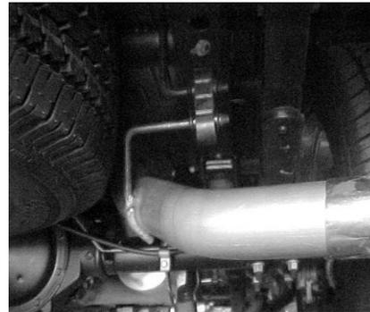
INSTALL OVER-AXLE TAILPIPE # D INTO MUFFLER 1 1/2" - 2", INSERT WELDED HANGER INTO RUBBER GROMMET, ROTATE PIPE TO PROPER ANGLE.
