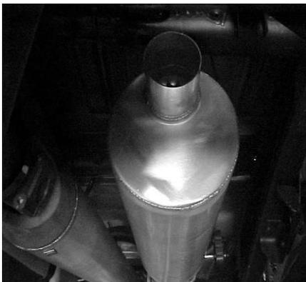
INSTALL MUFFLER # C ONTO HEADPIPES 1 1/2"-2". USE CLAMPS # G TO SECURE OUTLET OF MUFFLER, IT SHOULD BE AT THE 12 O'CLOCK POSITION. USE A JACKSTAND TO SUPPORT MUFFLER.
