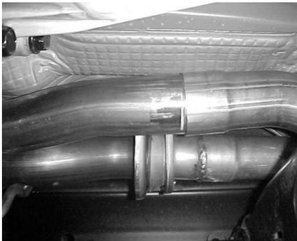
INSTALL PASS. SIDE HEADPIPE # A ONTO FACTORY FLANGE USING THE HARDWARE # H. INSERT WELDED HANGER INTO RUBBER GROMMET. DO NOT TIGHTEN. NEXT INSTALL DR. SIDE HEADPIPE # B ONTO FACTORY PIPE USE CLAMP # G TO SECURE, DO NOT TIGHTEN.
