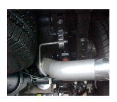
INSTALL OVER-AXLE TAILPIPE # D INTO MUFFLER 1 ½" – 2", INSERT WELDED HANGER INTO RUBBER GROMMET, ROTATE PIPE TO PROPER ANGLE.
