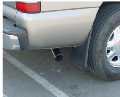
INSTALL THE STAINLESS STEEL TIP NOW, FIRMLY TIGHTEN EVERYTHING ALL CLAMP, HANGERS, BOLTS, FLANGE. TO CLEAN TIP USE ANY STAINLESS CLEANER WITH A SCOTCH BRITE PAD.
