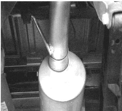
NEXT CONNECT THE MUFFLER TO THE HEADPIPE 1 1/2" TO 2" USING CLAMP #E. TO SECURE MUFFLER TO PIPE, USE JACKSTANDS TO SUPPORT THE MUFFLER. THE OUTLET OF THE MUFFLER WILL BE AT APPROXIMATELY 11 O'CLOCK. THE MUFFLER INLET IS LOOKING INTO THE LOUVERS. DO NOT TIGHTEN.
