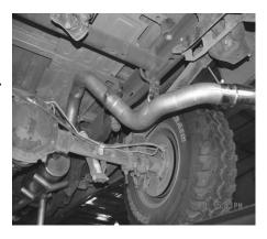
INSTALL OVERAXLE TAILPIPE #D INTO MUFFLER. INSERT WELDED HANGER INTO RUBBER GROMMET. USE CLAMP #F TO SECURE PIPE TO MUFFLER, DO NOT TIGHTEN.
