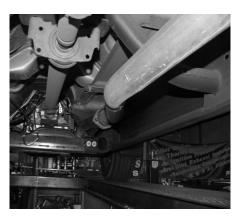
TO REMOVE THE STOCK EXHAUST UN-BOLT IT FROM THE 2-BOLT FLANGE LOCATED JUST BEHIND THE FACTORY Y-PIPE. YOU WILL NEED TO RE-USE THE FACTORY BOLTS. NOW CUT OFF YOUR STOCK TAILPIPE JUST BEHIND THE MUFFLER AND REMOVE. LEAVE ALL RUBBER GROMMETS ON THE HANGERS. USE WD-40 TO AID IN REMOVAL OF THE
