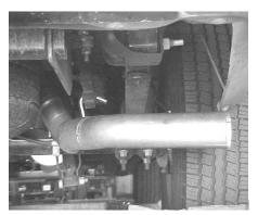
INSERT EXITPIPE #E ONTO TAILPIPE. INSERT WELDED HANGER INTO RUBBER GROMMET. USE CLAMP #F TO SECURE EXITPIPE TO TAILPIPE, DO NOT TIGHTEN. ROLL THE EXIT PIPE UNTIL IT IS LEVEL.
