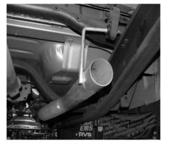
INSTALL HEADPIPE #A ONTO STOCK FLANGE USING THE FACTORY BOLT TO SECURE IT. DO NOT TIGHTEN. NEXT INSTALL HEADPIPE #B ONTO #A HEADPIPE #B ONTO #A HEADPIPE YOU WILL USE CLAMP #F TO SECURE HEADPIPE #A TO #B, DO NOT TIGHTEN. INSERT WELDED HANGER INTO RUBBER GROMMET.
