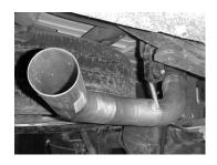
Install exit pipe #D onto the tailpipe.
