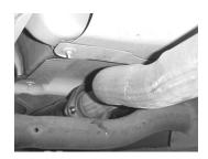
Lay out the exhaust on the floor so it looks like the drawing and compare parts with manual. To remove the stock exhaust, remove it from the factory 2-bolt flange located in front of the muffler. Do not disguard the factory hardware you will reuse them. Leave all rubber grommets in place. Use WD-40 to aid in removal of exhaust and hangers. Cut off your
